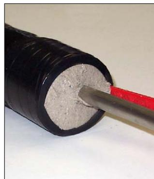
✓ Weatherproof seals must be installed at each end of the tubing bundle. Select the end seal kit designed for the maximum exposure temperature.
