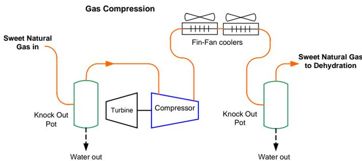
Post compression the wet natural gas must be dried (dehydrated), reducing water vapor content to a level of less than 1.0 ppmv. The middle bed of each drier and its outlet will require trace moisture measurement.
