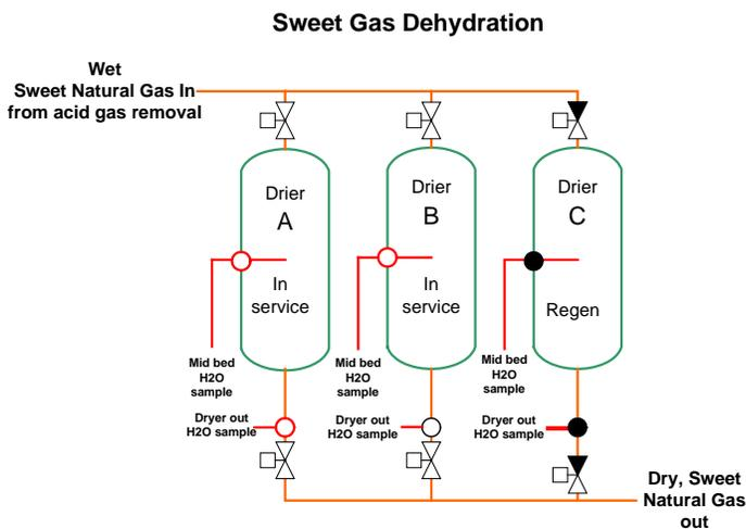
The Trace Moisture sample points are at approximately 54 bar G, the sample is usually transported at process pressure to AlO<sub>3</sub> moisture sensor probes. The sample transport line should be heat traced to maximum ambient temperature + 10 °C to minimize diurnal temperature effects. We have a trace moisture
