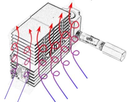
Incorrectly mounted heater does not allow for proper airflow.
