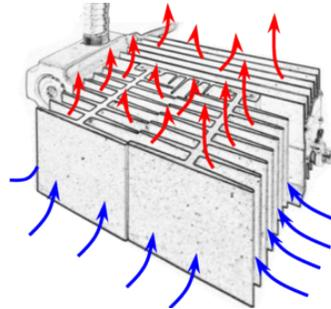
Fins must be vertical to allow for airflow.
