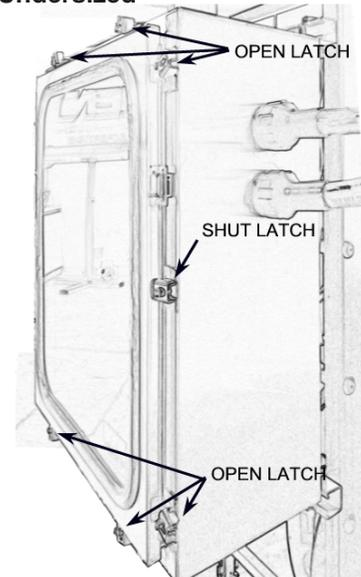
Latches that are left open can increase the heat loss by 20 – 30%.
