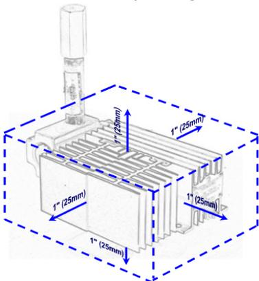
Allow a minimum of 1" (25mm) on all sides, top and bottom of heater for sufficient airflow.
