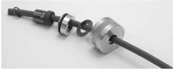
5. Begin 3/4" (20 mm) from the mark made where the cable enters the fitting and remove the outer cable jacket to expose the grounding braid. Be careful not to damage the braid.
