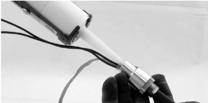
15. Using heat gun, heat insert assembly to about 260°F. (127°C.) for several minutes until thermoset potting material hardens. (It will take about two minutes to harden at room temperature applying 260°F heat.)
