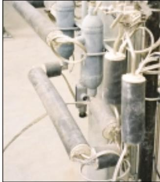
**X** Unsealed bundle ends, splices and terminations allow moisture to be absorbed by the insulation. Wet insulation degrades the bundle two ways: by reducing the insulating properties and secondly by releasing water soluble chlorides which may contribute to chloride stress corrosion of stainless steel process tubes.
