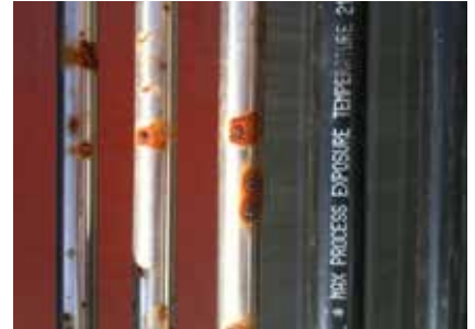
Localized corrosion due to weld slag adhesion on 2507 Super Duplex tubes.
