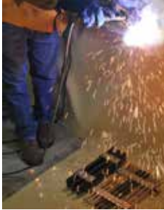
Weld slag adheres to all metal alloys including high CRA 2507 Super Duplex (UNS S32750) and creates localized corrosion.
