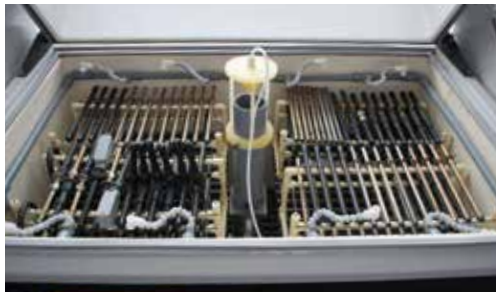
Protected 316 vs. Exposed Tube
