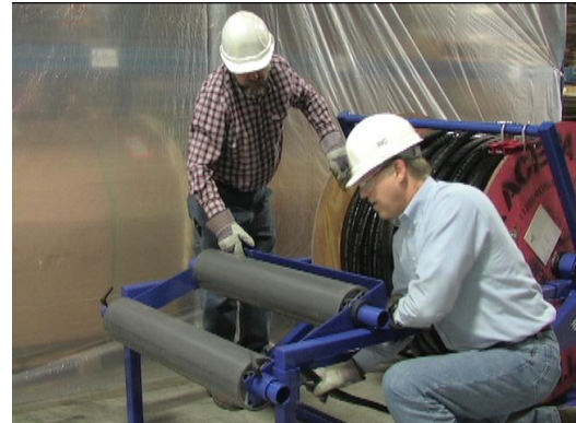
Thread bundle through rollers.
