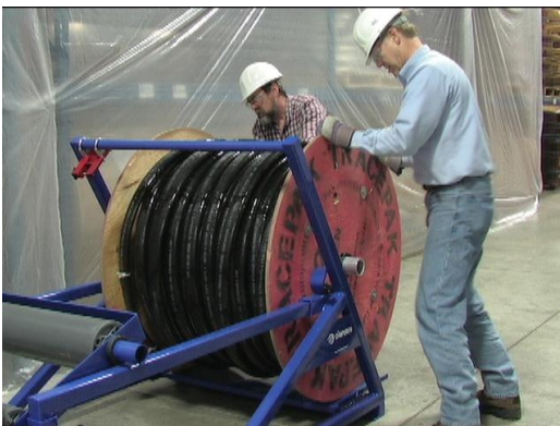
Use ramp to load spool and install safety pins.
